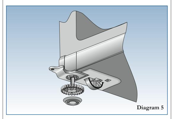
Tilt the product back and remove the levelling foot circular base insert from the front levelling feet, a small flat blade screw driver can be used.
