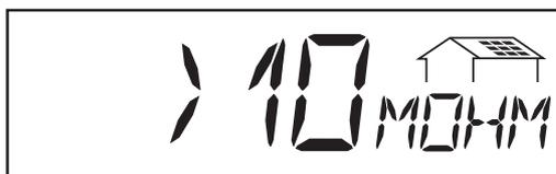
**Insulation resistance** of the photovoltaic system (MOhms)
