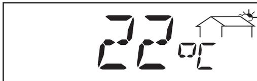
\* **Ambient temperature** (°C; °C; can be changed to °F in the setup menu; temperature sensor no. 2; sensor card option)
