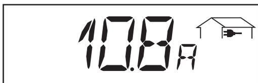
**Current fed in ...** Current (in amperes) currently being fed into the mains ... from the master power module phase
