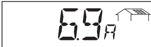
**Module current** ... Current that is being supplied at present by the solar modules ... (amperes)
