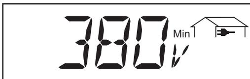
**Minimum mains voltage** ... smallest mains voltage (V) measured during the time in question ... from the master power module phase ... Measured value applies to the three-phase mains circuit (Example: 220 V \* 1.73 = 380 V)
