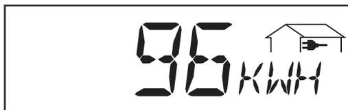
**Energy fed in** ... Energy fed into the mains over the period of time in question (kWh / MWh)
