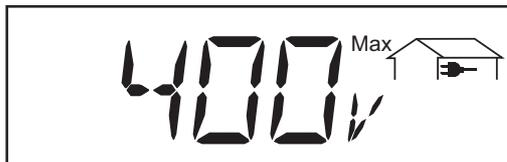
**Maximum mains voltage** ... largest mains voltage (V) measured during the time in question ... from the master power module phase ... Measured value applies to the three-phase mains circuit (Example: 231 V \* 1.73 = 400 V)
