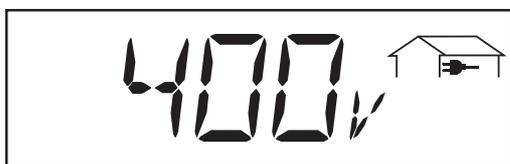
**Mains voltage** (volts) ... from the master power module phase ... Measured value applies to the three-phase mains circuit
