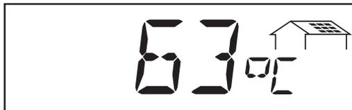
\* **Module temperature** ... Temperature at the solar modules (°C; can be changed to °F in the setup menu; temperature sensor no. 1; sensor card option)
