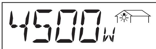
\* **Power taken out of the mains** ... Current consumption (in watts; optional sensor card)
