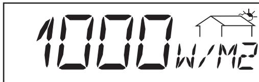
\* **Insolation** ... Insolation power coming down on each square metre (watts/m²; optional sensor card)
