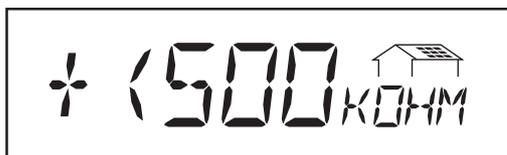
Example of display for positive potential (polarity sign „+“):
