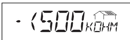
Example of display for negative potential (polarity sign „-“)
