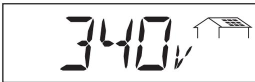
**Module voltage ...** Voltage (in volts) currently present at the solar modules
