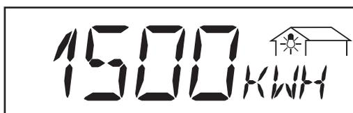
\* **Energy recorded by the consumption meter** ... energy consumed during the time in question (kWh / MWh; optional consumption sensor)
