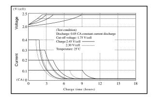
In order to fully utilize the characteristics of SLA batteries, constant-voltage charging is recommended.
