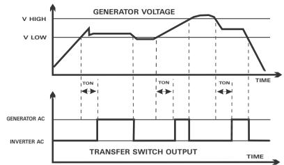
Ton = On Delay timer is selectable at 30 or 120 seconds.
