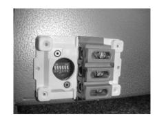
ENSURE POWER IS DISCONNECTED BEFORE ADJUSTING DIP SWITCHES.
