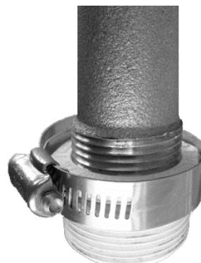
Hose clamp reinforcing a plastic reducer bushing
