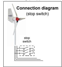
We recommend installing a 'stop' switch which should be more correctly thought of as a 'parking' switch. Just as the parking brake in a car should not be relied on to stop a car at high speed, so the parking switch of the Ampair wind turbine should not be relied on to stop the rotor disc in high winds. Instead it is best to apply it before the arrival of very high winds, or if needing to ensure that the rotor does not move in low winds (e.g. when approaching the rotor for maintenance).
