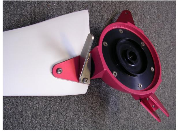
The holes in the blades are a deliberately tight fit and it may be necessary to turn the fasteners as they are inserted. First loosely fit all the nylock nuts by hand, then fully tighten with a spanner. Finally, recheck the tightness of all the nuts.
