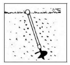
**Ground anchors:** These should be suitable eyebolts fixed in the ground and in line with the guys. Anchors in soft earth may require concrete blocks or 'dead men'. Gravel or clay soils require "auger" type anchors (see inset picture) and rocky ground may need drilling and expanding rock anchors. Only the eye should be visible above ground. Avoid waterlogged soils which have poor holding properties. Install anchor below the frost level or otherwise 'frost heave' will eject them.
