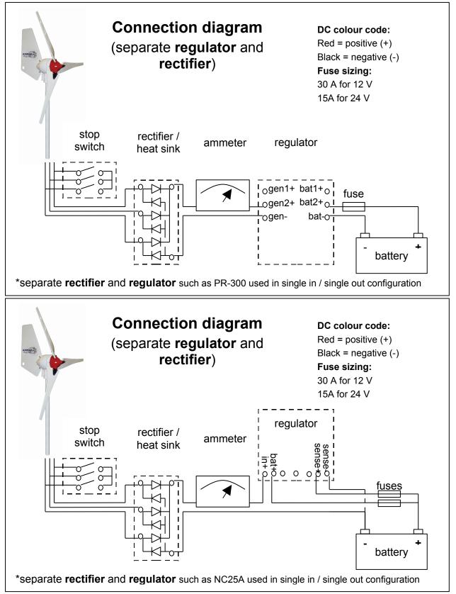
If the Pacific 300 wind turbine is connected on the load side of the battery isolator switch, it may damage electrical equipment. Under these conditions it is possible to run the wind turbine whilst the battery is isolated, but this can subject the system to excess voltage.
