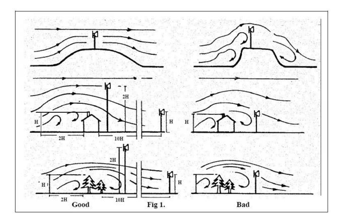
**WARNING:** Before a wind turbine is installed in an excessively windy location, the operators must satisfy themselves that the site is suitable. It may be necessary to log site wind speed and direction data at various heights prior to installing the machine.
