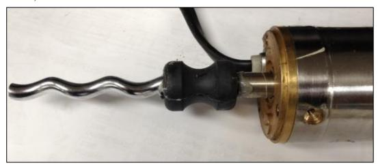
Step 5 Using an 8mm spanner, unfasten the nuts from the U-bolts on the pump outlet. Separate the metal retaining plate from the outlet and remove the rubber stator from the brass bush. Inspect the condition of the stator and replace as required.
