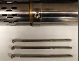
Step 3 Gently pull apart the pump outlet, shroud and motor ensuring that the power cable is not damaged.
