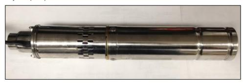
Step 2 Using a 10mm spanner, unfasten each of the three retaining bolts joining the pump outlet, shroud and motor together and set aside.
