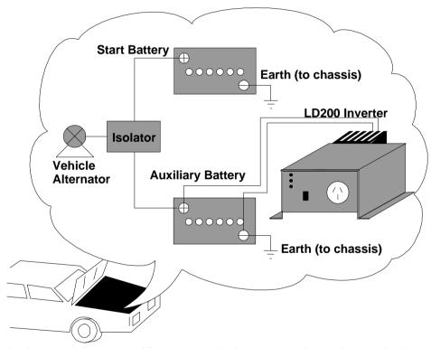
By incorporating an auxiliary battery in the manner above, the starting battery should remain charged for vehicle starting (see your auto electrician). The LD200 has sufficient battery cable length to allow it to sit underneath the vehicle whilst in use. If the ground is wet, place the LD200 on a waterproof liner.
