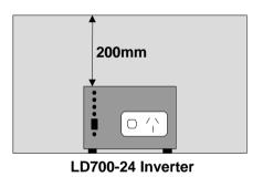
Please leave a clearance of 200mm on all sides and top of the Inverter. The LD700-24 must be installed in a dry, cool, dust-free environment. It is recommended that the inverter be placed as far from any radio receivers as possible.
