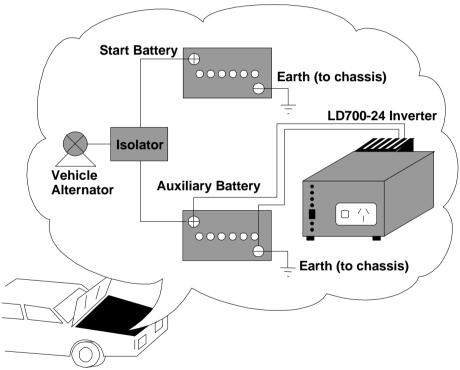
By incorporating an auxiliary battery in the manner above, the starting battery should remain charged for vehicle starting (see your auto electrician). The LD700-24 has sufficient battery cable length to allow it to sit underneath the vehicle whilst in use. If the ground is wet, place the LD700-24 on a waterproof liner.
