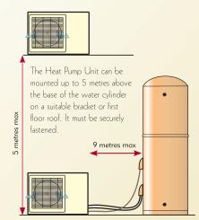
The Heat Pump Unit is supplied with 2 metres of pre-charged connecting lines. Additional kits of up to 7 metres of pre-charged and insulated tubes are available depending on installation.
