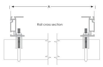
Distance between rails' outer edges (A) equals distance between module mounting-hole centers minus 1 inch (2.5 cm).
